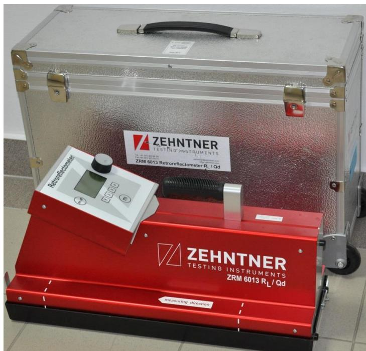
The Zehntner-retroreflektometer ZRM 6013 measures the night visibility (RL) of road markings as seen by a vehicle driver driving with dipped headlights. The illumination simulates the dipped headlights of a vehicle. The day visibility (Qd) of road markings under typical or average daylight or under street lighting is measured with diffused illumination. This makes an objective determination.
